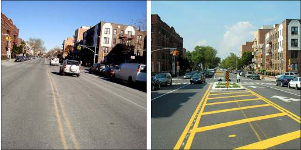
Figure 17: Road Diet - Image Source: FHWA
